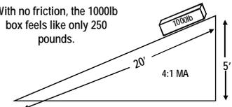
**Percentage Of Load Based on Slope w/o Friction**
