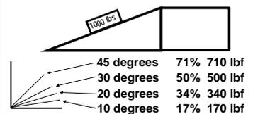
This is the force required to push object up the ramp as a percent of its weight.
