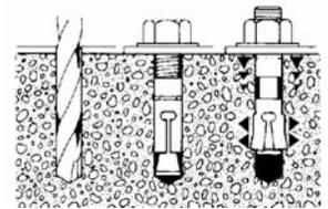
Have Reduced Capacity in Cracked Concrete
