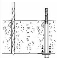
**Bolt or rod with double nuts and a large washer**
