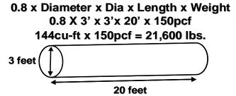
• For a Hollow Round Object, like a Pipe, we can use Method 1 - find the weight of the solid round, then subtract the weight of the hole
