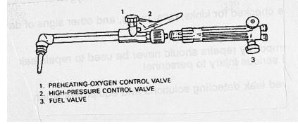
• Machine torches: A torch equipped with valves controlling oxygen, fuel gas, and cutting oxygen with tubes encased in a body with a head to accept the cutting tip.
